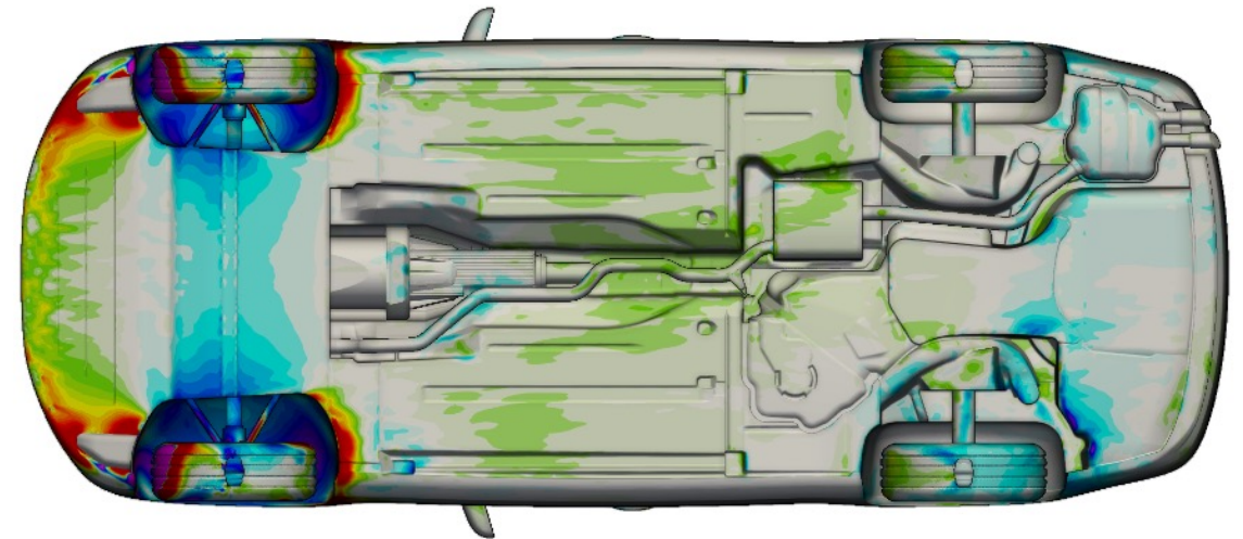
RUN007 minus RUN004 As R004 but with front tyre deflectors
